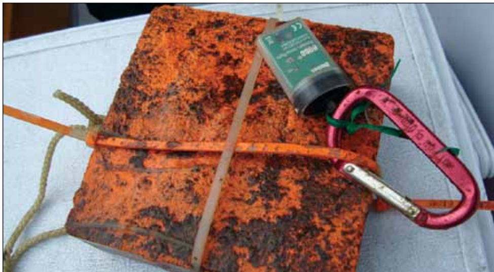
Hobo temperature and light logger after several months in the water.
