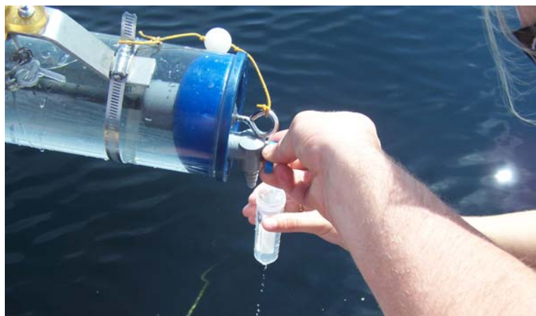
An intern pours off a sample from a deep water grab to be analyzed later for phosphorus concentration.
