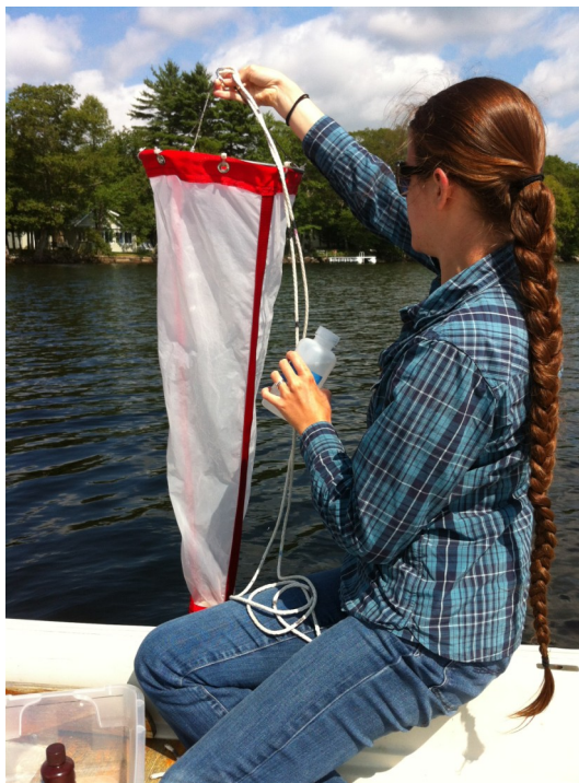
Collecting a sample using a plankton net.
