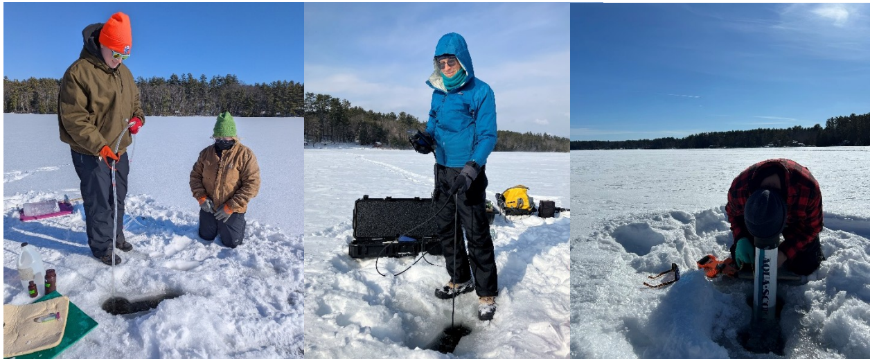
Sam and Morgan collecting water sample with core tube (left), Ben using the sonde (middle), and Tim measuring Secchi depth (right)
